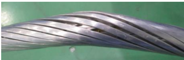
Strand opening due to sharp "local" overbending
