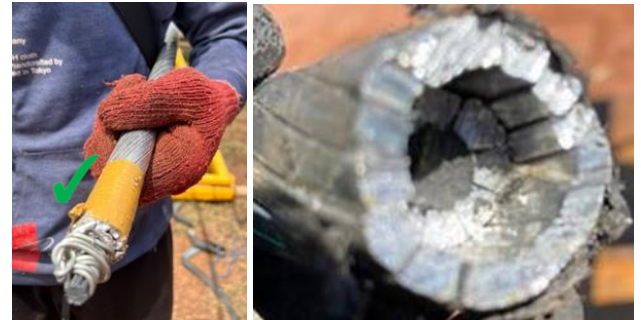
CFCC core can slip inside aluminum layer by tension stringing
