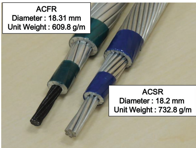
Figure 3. External appearance of aluminum conductor steel reinforced (ACSR) with a cross-sectional area of 160 mm 2 , and aluminum conductor fiber reinforced (ACFR) with a similar diameter.
