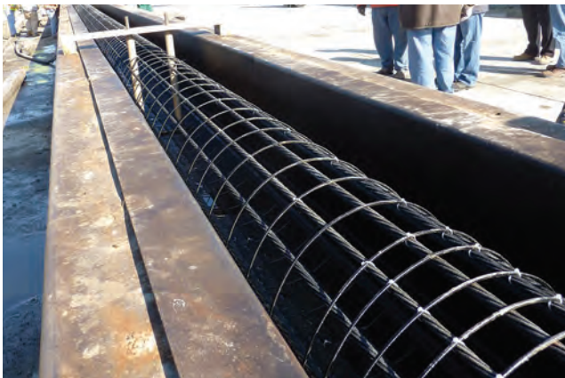
Prestressing bed with carbon-fiber-composite cable strands/spirals for piles for the Nimmo Parkway bridge in Virginia.
