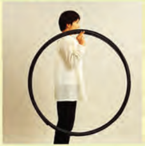
CFCC 1X7 \phi 15.2mm (0.6in) (Pre-tensioning)
