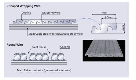
This S-shaped wrapping wire prevents cracking of coating by mean of the effect of interlocking of turns. The adoption of coating agent having an excellent elongation performance prevents from cracking due to expansion of cables and at the same time prevents the infiltration of rain water and others.
